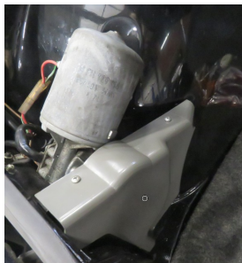
Gray cover on lifting lights relay
